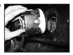
5. From the front of the vehicle, check to make sure O-rings are properly seated between the Euro Guards and the bumper.
